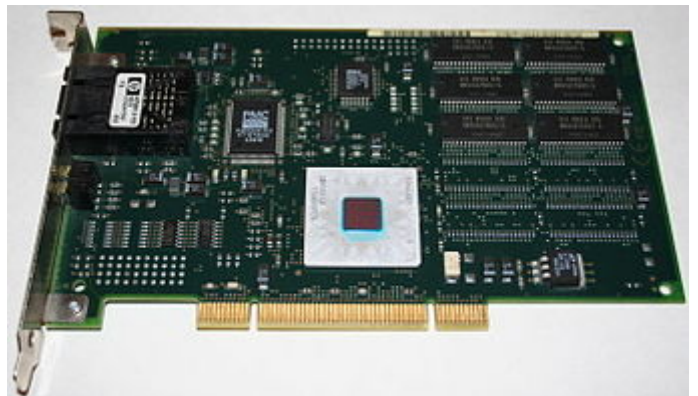
IBM Turboways ATM 155 PCI network interface card
