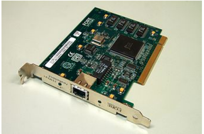
Marconi ForeRunnerLE 25 ATM PCI network interface card
