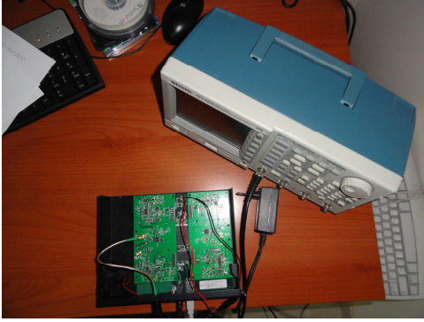
Fig. 4. The hardware necessary to implement a GSM BTS.
