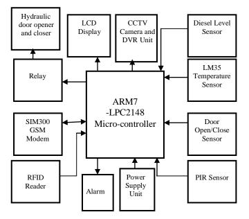
The whole site room is under the cover of CCTV camera. The site room includes door open/close sensor. Whenever any person enters the room the message is sent to the site admin and CCTV camera turns ON. The system includes a temperature sensor within the Site. If the site temperature rises above the maximum allowed value, the system automatically opens the site door and sends this information message to technician
