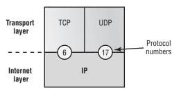
In this example, the protocol field tells IP to send the data to either TCP port 6 or UDP port 17 (both hex addresses). However, it will only be UDP or TCP if the data is part of a data stream headed for an upper-layer service or application. It could just as easily be destined for ICMP (Internet Control Message Protocol), ARP (Address Resolution Protocol), or some other type of Network layer protocol.
