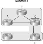
Partial mesh with full connectivity using subinterfaces
