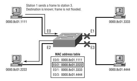
In this figure, there are four hosts attached to a switch. When the switch is powered on, it has nothing in the MAC address table.
