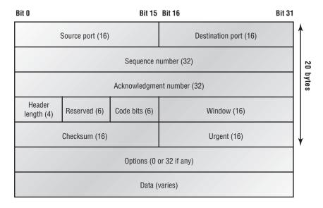
The TCP header is 20 bits long. You need to understand what each field in the TCP segment is. The TCP segment contains the following fields:
