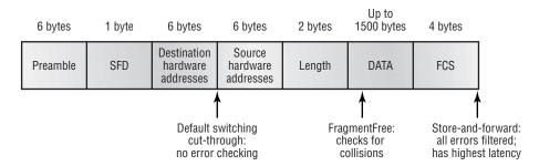
FIGURE 2.6 Different switching modes within a frame
