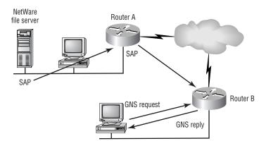
FIGURE 8.2 Remote IPX clients on a serverless network
