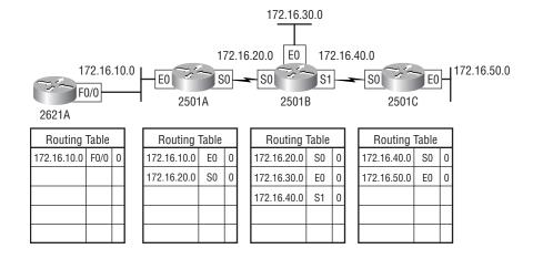
As shown in Figure 5.6, each router has only the directly connected networks in each routing table. Each router sends its complete routing table out to each active interface on the router. The routing table of each router includes the network number, exit interface, and hop count to the network.
