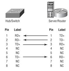
You can determine that the wiring is a straight-through cable by holding both ends of the UTP cable side by side and seeing that the order of the wires on both ends is identical.
