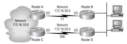
Since network 172.16.30.0 is a T1 link with a bandwidth of 1.544Mbps, and network 172.16.20.0 is a 56K link, you would want the router to choose the T1 over the 56K link. However, since hop count is the only metric used with RIP routing, they would both be seen as equal-cost links. This is called pinhole congestion.
