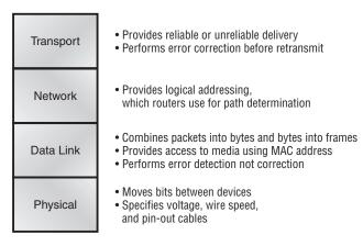
The four bottom layers define how data is transferred through a physical wire or through switches and routers, and how to rebuild a data stream from a transmitting host to a destination host's application.
