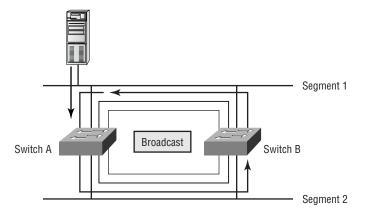
2. A device can receive multiple copies of the same frame since the frame can arrive from different segments at the same time. Figure 2.3 shows how multiple frames can arrive from multiple segments simultaneously.
