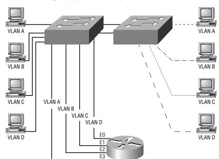
FIGURE 6.3 Switches removing the physical boundary
