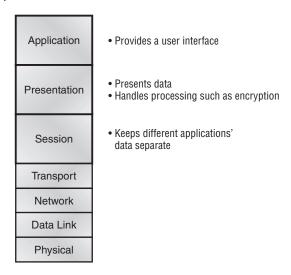
In Figure 1.1, you can see that the user interfaces with the computer at the application layer, and also that the upper layers are responsible for applications communicating between hosts. Remember that none of the upper layers know anything about networking or network addresses. That is the responsibility of the four bottom layers, which are shown in Figure 1.2.
