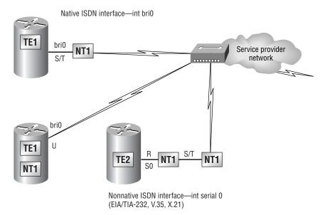
FIGURE 10.7 ISDN BRI reference points and terminal equipment
