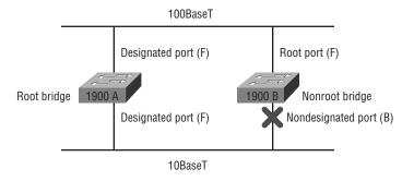
Ports determined to have the lowest-cost path to the root bridge are called designated ports. The other port or ports on the bridge are considered nondesignated and will not send or receive traffic, which is called blocking mode.
