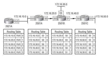
The routing tables in each router keep information regarding the network number, the interface to which the router will send packets out to get to the remote network, and the hop count or metric to the remote network.
