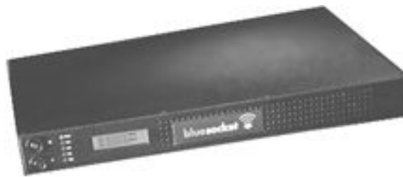
FIGURE 4.20 An enterprise wireless gateway installed on a network
