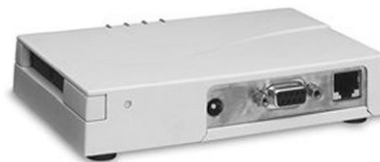
FIGURE 4.14 A sample Ethernet and serial converter
