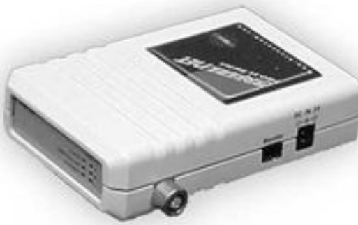
FIGURE 4.12 A wireless workgroup bridge installed on a network
