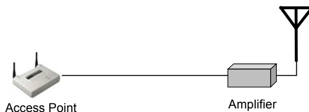
FIGURE 5.23 RF amplifier placement in the wireless LAN system
