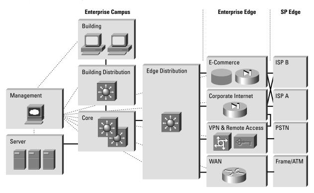
While it is true that most existing enterprise networks cannot be easily dissected into clear-cut modules, this approach provides a guide for implementing different security functions throughout the network. The authors do not expect network engineers to design their networks identical to the SAFE implementation, but rather use a combination of the modules described and integrate them into the existing network.
