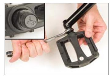
Note: You will damage the threads in the crank arms if you thread the wrong pedal into the wrong crank arm.
