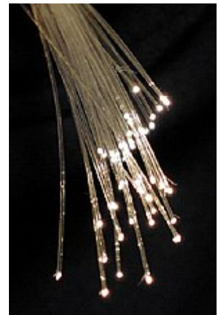
Fiber optic cables are used to transmit light from one computer/network node to another
