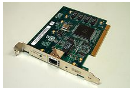
An ATM network interface in the form of an accessory card. A lot of network interfaces are built-in.
