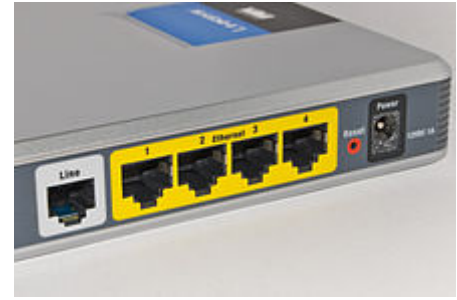
A typical home or small office router showing the ADSL telephone line and Ethernet network cable connections
