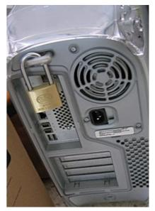
While most aspects of computer security involve digital measures such as electronic passwords and encryption, physical security measures such as metal locks are still used to prevent unauthorized tampering.
