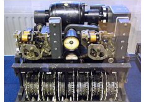
German Lorenz cipher machine, used in World War II to encrypt very-high-level general staff messages
