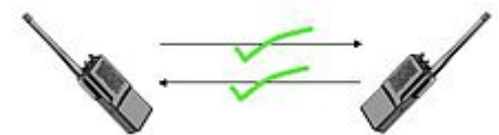
A simple illustration of a full-duplex communication system. Full-duplex is not common in handheld radios as shown here due to the cost and complexity of common duplexing methods, but is used in telephones , cellphones and cordless phones .
