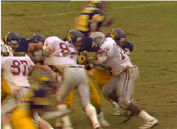
Single B-frame IP packet loss (1 frame affected)
