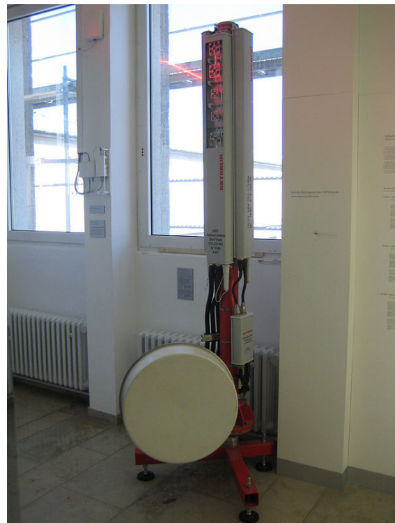
GSM cell site antennas in the Deutsches Museum, Munich, Germany
