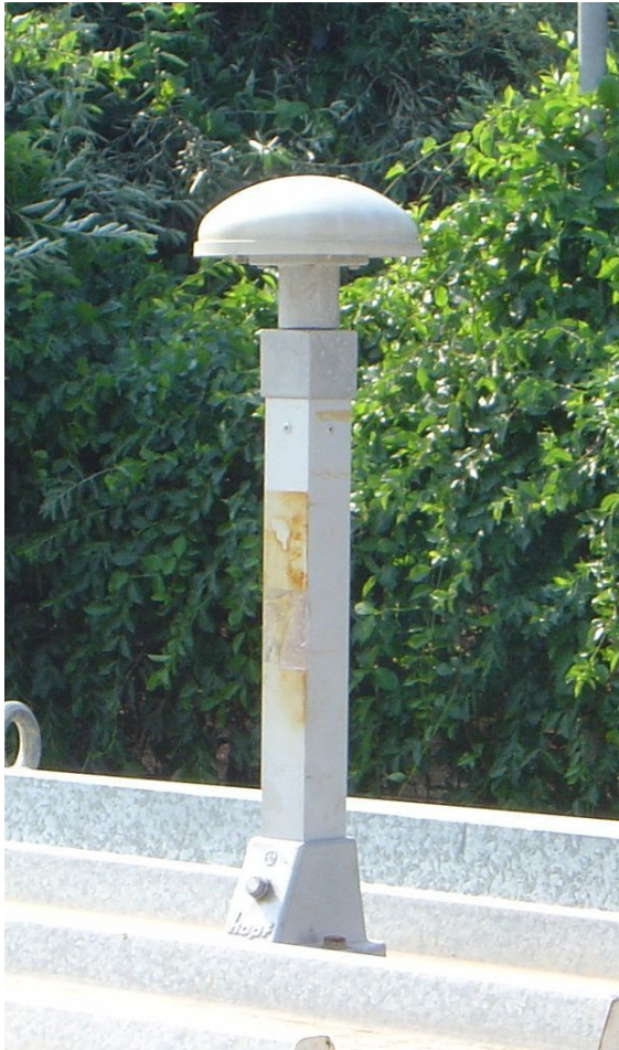
This antenna is mounted on the roof of a hut containing a scientific experiment needing precise timing.
