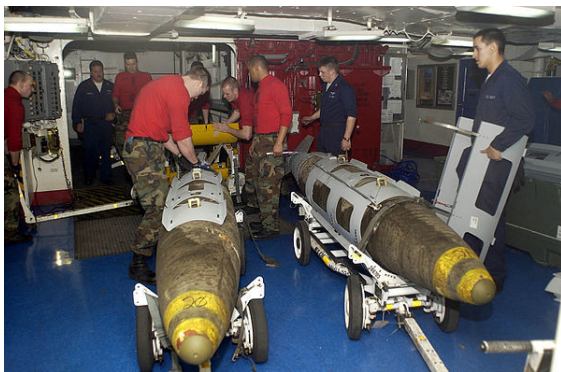
Attaching a GPS guidance kit to a dumb bomb, March 2003.
