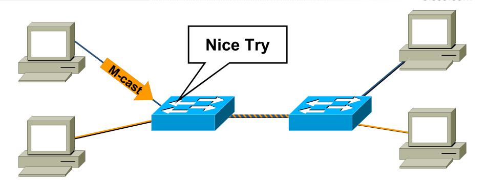
Send random Ethernet multicast frames to a switch interface attempting to get frames to another VLAN
