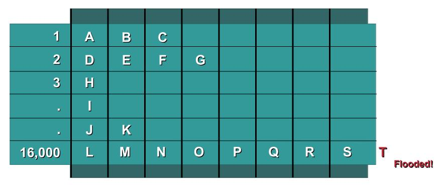
• 63 bits of source (MAC, VLAN, misc) creates a 17 bit hash value If the value is the same there are 8 buckets to place CAM entries, if all 8 are filled the packet is flooded
