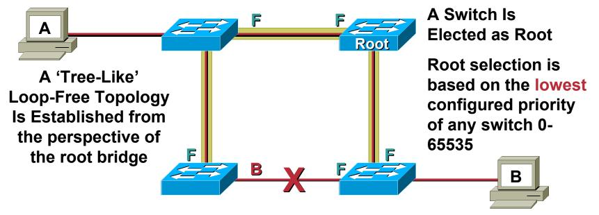
STP is very simple. Messages are sent using Bridge Protocol Data Units (BPDUs). Basic messages include: configuration, topology change notification/acknowledgment (TCN/TCA); most have no "payload"
