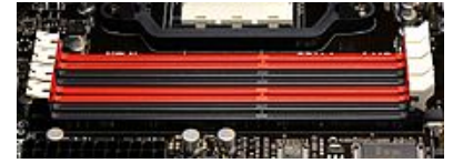
Motherboards often use color coded slots to indicate which slot corresponds to which RAM channel
