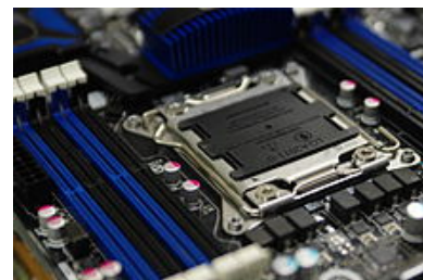
Some motherboard CPU sockets come with a plastic protector. This should be removed before the CPU is inserted, and saved for later.
