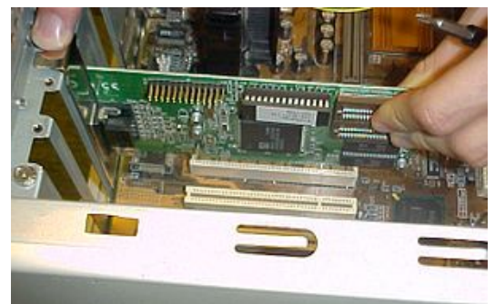
Insert the card into a matching slot on the motherboard.
