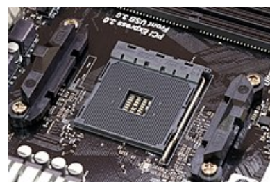
An AM4 socket for AMD processors
