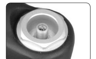
Cover cap and valve of the air spring system side of the fork
