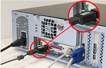
*A connected hardware-based keylogger*
