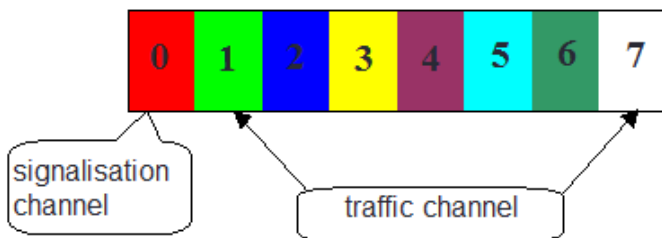
TDMA Frame for GSM
