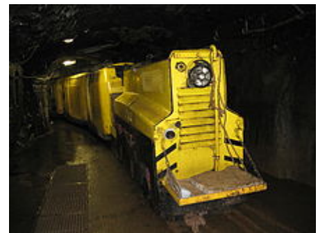
Mantrip used for transporting miners within an underground mine
