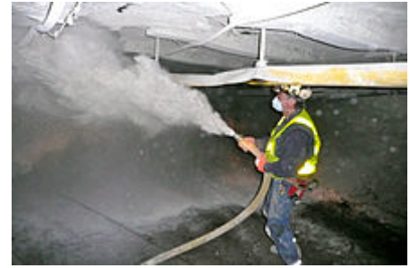
A coal miner in West Virginia spraying rockdust to reduce the combustible fraction of coal dust in the air.
