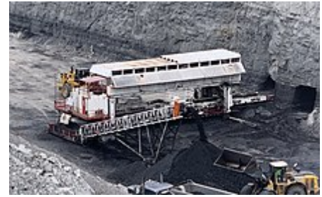
Coalburg Seam highwall mining at ADDCAR 16 Logan County WV
