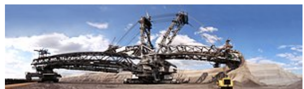
The Bagger 288 is a bucket-wheel excavator used in strip mining . It is also one of the largest land vehicles of all time.
