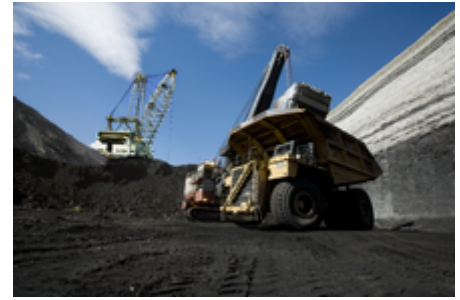
A Bucyrus Erie 2570 dragline and CAT 797 haul truck at the North Antelope Rochelle opencut coal mine
