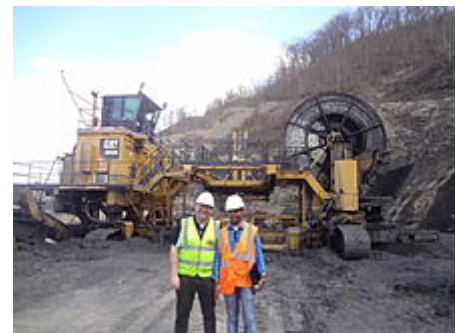
Caterpillar Highwall Miner HW300 – Technology Bridging Underground and Open Pit Mining
