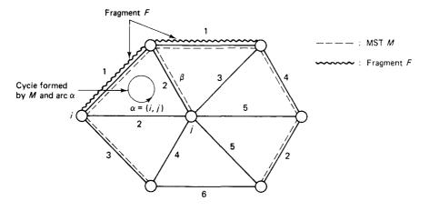
**Figure 5.25** Proof of Proposition 1. The numbers next to the arcs are the arc weights. F is a fragment which is a subtree of an MST M. Let  $\alpha$  be a minimum weight outgoing arc from F not belonging to M. Let  $\beta \neq \alpha$  be an arc that is outgoing from F and simultaneously belongs to M and to the cycle formed by  $\alpha$  and M. Deleting  $\beta$  from M and adding  $\alpha$  in its place forms another MST M'. When F is extended by  $\alpha$ , it forms a fragment.
