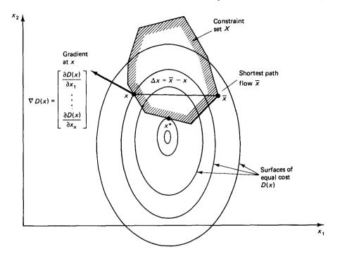
**Figure 5.68** Finding the feasible descent direction  $\Delta x = \overline{x} - x$  at a point x in the Frank–Wolfe method.  $\overline{x}$  is the shortest path flow (or extreme point of the feasible set X) that lies farthest out along the negative gradient direction  $-\nabla D(x)$ .
