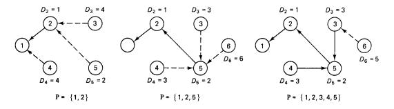
Figure 5.35 Example using the Bellman–Ford and Dijkstra algorithms.
