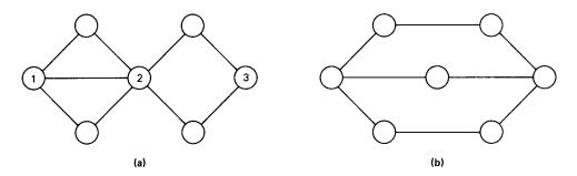
**Figure 5.56** Illustration of the definition of k-connectivity. In graph (a), nodes 1 and 2 are 6-connected, nodes 2 and 3 are 2-connected, and nodes 1 and 3 are 1-connected. Graph (a) is 1-connected. Graph (b) is 2-connected.
