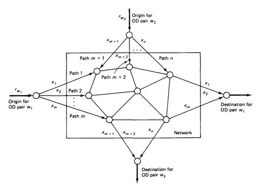
**Figure 5.51** Schematic representation of a network with two OD pairs  $w_1$  and  $w_2$ . The paths of the OD pairs are  $P_{w_1} = \{1, 2, ..., m\}$  and  $P_{w_2} = \{m + 1, m + 2, ..., n\}$ . The traffic inputs  $r_{w_1}$  and  $r_{w_2}$  are to be divided into the path flows  $x_1, ..., x_m$  and  $x_{m+1}, ..., x_n$ , respectively.
