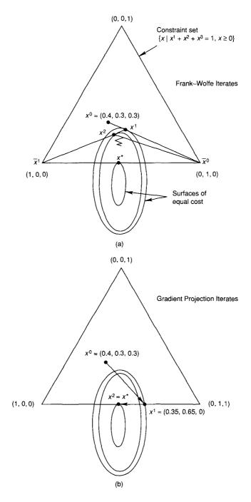
**Figure 5.71** Iterates of (a) the Frank–Wolfe and (b) the gradient projection method for the example of the preceding section. The gradient projection method converges much faster. It sets the flow  $x_3$  to the correct value 0 in one iteration and (because the Hessian matrix here is diagonal and the cost is quadratic) requires one more iteration to converge.
