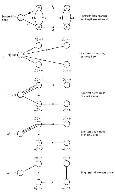
**Figure 5.31** Successive iterations of the Bellman–Ford method. In this example, the shortest ( $\leq h$ ) walks are paths because all arc lengths are positive and therefore all cycles have positive length. The shortest paths are found after N-1 iterations, which is equal to 4 in this example.
