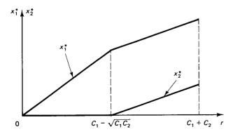
**Figure 5.62** Optimal path flows for the routing example. When the traffic input is low, only the high-capacity link is used. As the input increases beyond the threshold  $C_1 - \sqrt{C_1C_2}$ , some traffic is routed on the low-capacity link.
