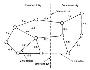
**Figure 5.55** Illustration of the cut saturation method for performing a branch exchange heuristic. The number next to each arc is the link utilization. Links of high utilization are temporarily removed until the network separates into two components,  $N_1$  and  $N_2$ . A link is then added that connects a node in  $N_1$  with a node in  $N_2$  while a link of low utilization is deleted.
