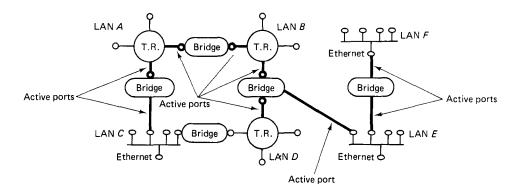
**Figure 5.16** Illustration of spanning tree in a network of LANs interconnected with bridges. The spanning tree consists of a set of bridge ports (called active), which connect all LANs into a network without cycles. Only active ports are used for routing packets and thus there is a unique route connecting a pair of LANs. For example, a packet of a station connected to LAN C will go to a station in LAN E through LANs A and B.
