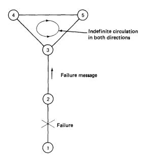
**Figure 5.44** Example of a form of flooding where the transmission of messages never terminates. The rule is that a node that receives a message relays it to all of its neighbor nodes except the one from which the message was received. A failure of link (1. 2) is communicated to node 3. which triggers an indefinite circulation of the failure message along the loop (3,4,5) in both directions. This form of flooding works only if the network has no cycles.
