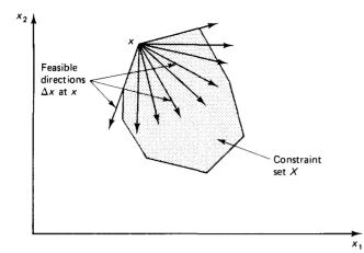
**Figure 5.63** Feasible directions  $\Delta x$  at a feasible point x.  $\Delta x$  is a feasible direction if changing x by a small amount along the direction  $\Delta x$  still maintains feasibility.
