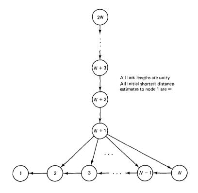
Figure 5.37 Example where the asynchronous version of the Bellman–Ford algorithm requires many more message transmissions than the synchronous version. The initial estimates of shortest distance of all nodes is  $\infty$ . Consider the following sequence of events, where all messages are received with zero delay:
