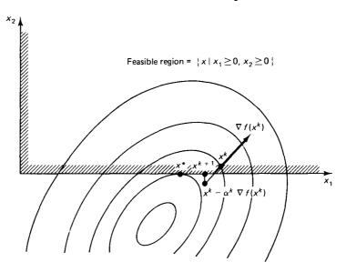
**Figure 5.70** Operation of the gradient projection method. A step is made in the direction of the negative gradient, and the result is orthogonally projected on the positive orthant. It can be shown that the step  $(x^{k+1} - x^k)$  is a descent direction [makes a negative inner product with  $\nabla f(x^k)$ ], and if the stepsize  $\alpha$  is sufficiently small, the iteration improves the cost [*i.e.*,  $f(x^{k+1}) < f(x^k)$ ].
