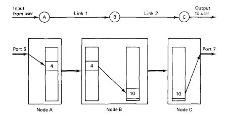
**Figure 5.13** Structure of TYMNET routing tables. For the virtual circuit on the path ABC, the routing table at node A maps input port 5 onto channel 4 on link 1. At node B, incoming channel 4 is mapped into outgoing channel 10 on link 2. At node C, incoming channel 10 is mapped into output port 7.
