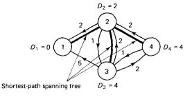
**Figure 5.33** Construction of a shortest path spanning tree. For every  $i \neq 1$ , a neighbor node  $j_i$  minimizing  $d_{ij} + D_j$  is selected. The tree of the  $N - 1 \arccos (i, j_i)$  defines a set of shortest paths.
