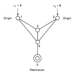
**Figure 5.72** The network, for the example, where node 5 is the only destination and there are two origins, nodes 1 and 2.
