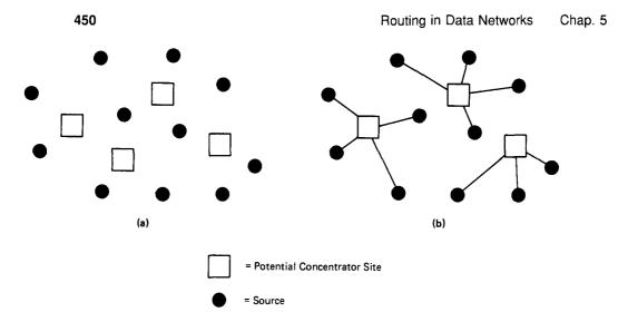
**Figure 5.60** (a) Collection of sources and potential concentrator locations. (b) Possible assignment of sources to concentrators.
