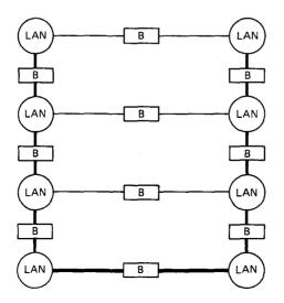
Figure 5.19 Example of inefficient spanning tree routing. The routing paths are good for origin LANs near the bottom of the figure but poor for origin and destination LANs near the top of the figure.
