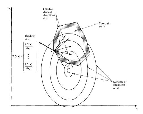
**Figure 5.64** Descent directions at a feasible point x form an angle greater than 90° with the gradient  $\nabla D(x)$ . At the optimal point  $x^*$ , there are no feasible descent directions.
