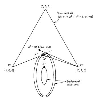
Figure 5.67 Successive iterates of the Frank–Wolfe method in the two-node, three-link example. Slow convergence is due to the fact that as the optimal solution  $x^*$  is approached, the directions of search tend to become orthogonal to the direction leading to the optimum.
