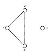
Figure 5.24 Graph with A = N - 1, which is both disconnected and contains a cycle.
