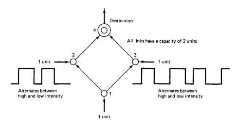
**Figure 5.52** Network of Example 5.6 where routing based on queue length information is beneficial. The traffic originating at nodes 2 and 3 alternates in intensity between 2 units and 0 units over large time intervals. A good form of routing gets information on the queue sizes at links (2,4) and (3,4) and routes the traffic originating at node 1 on the path of least queue size.
