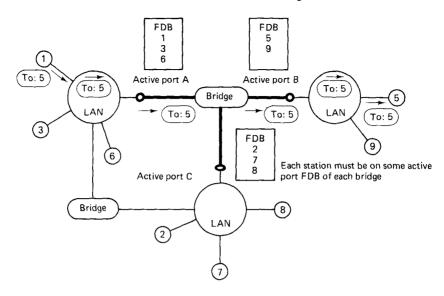
**Figure 5.17** Using forwarding databases (FDBs) to effect spanning tree routing. Each active port maintains an FDB, that is, a list of the stations with which it communicates. An active port, say A, checks the destination of each packet transmitted within its associated LAN. If the destination appears in the FDB of another active port of the same bridge, say B, the bridge broadcasts the packet on the LAN connected with port B.
