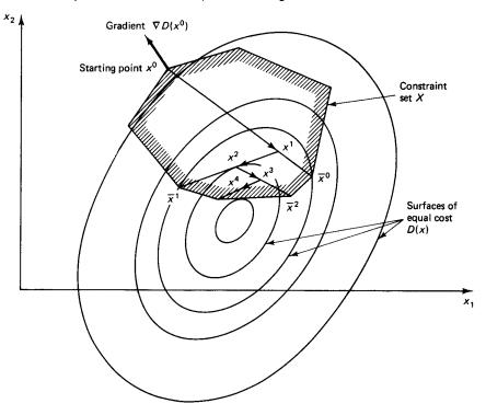
Figure 5.69 Successive iterations of the Frank–Wolfe method. At each iteration, a vertex of the feasible set (a shortest path flow) is found. The next path flow vector is obtained by a search on the line segment connecting the current path flow vector with the vertex.
