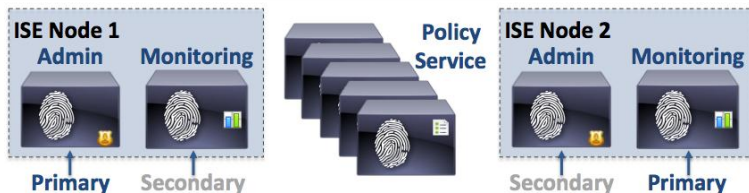
Figure 7 Distributed Deployment (2,000 to 10,000 Endpoints)
