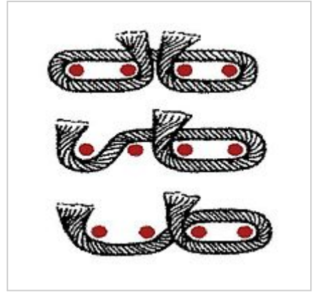
Variants of the "Jufti" knot woven around four warps
