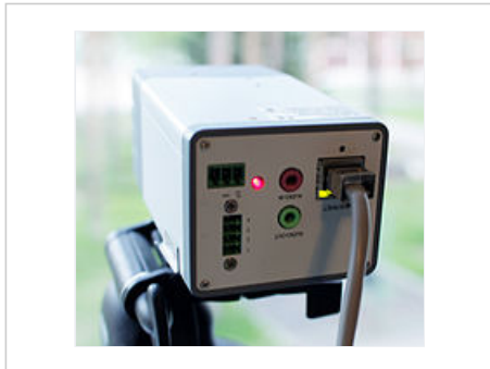
An IP camera powered by Power over Ethernet
