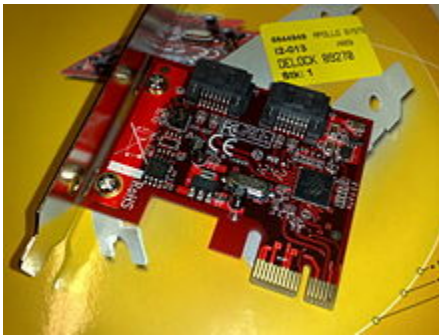
A SATA 3.0 controller that provides RAID functionality through proprietary firmware and drivers
