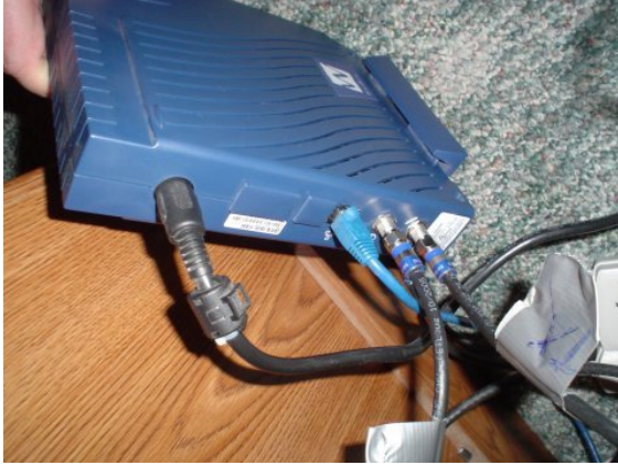
The back panel of a satellite modem, with coaxial connections for both incoming and outgoing signals, and an Ethernet port for connection
