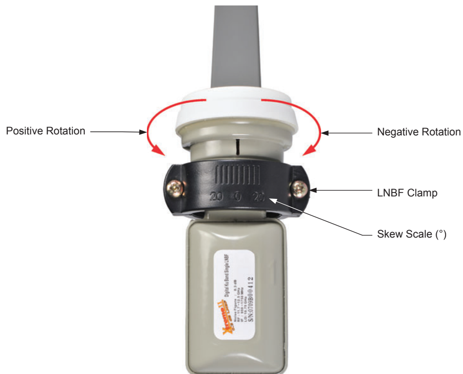
Figure 88. Skew adjustment for linear-polarization.
