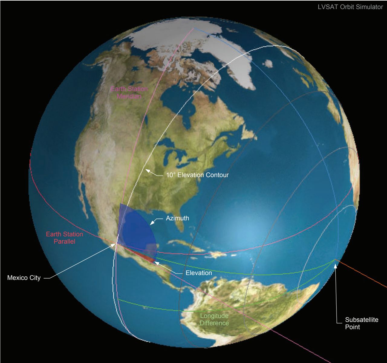
Figure 91. Determining the satellite longitude for 10° elevation to Mexico City.
