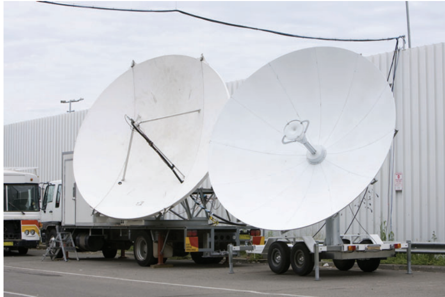
Figure 64. 5-meter transportable earth-station antennas.
