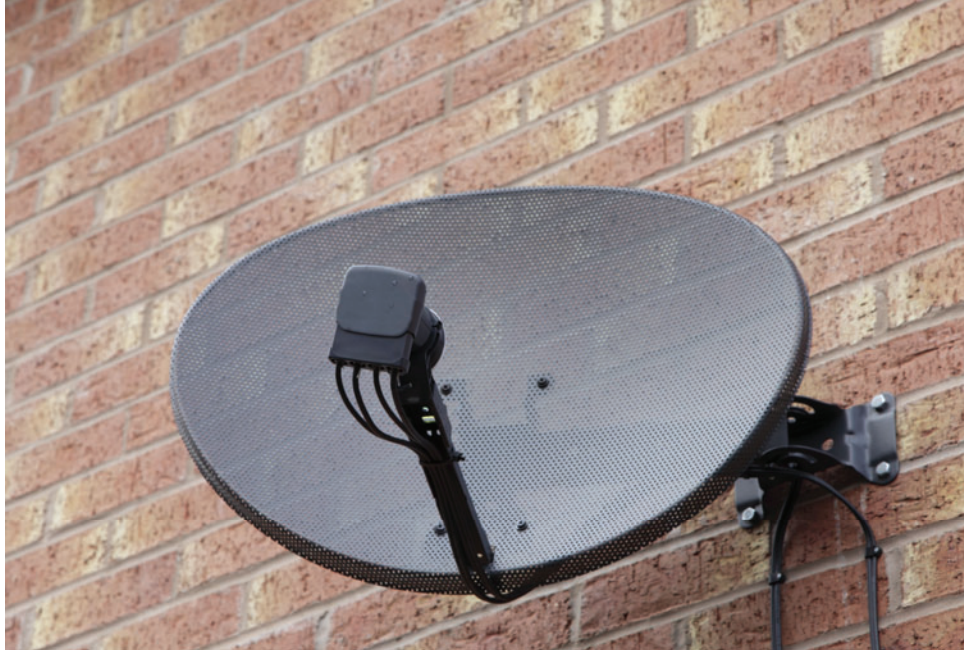
Figure 71. DBS antenna with an elliptical parabolic dish.
