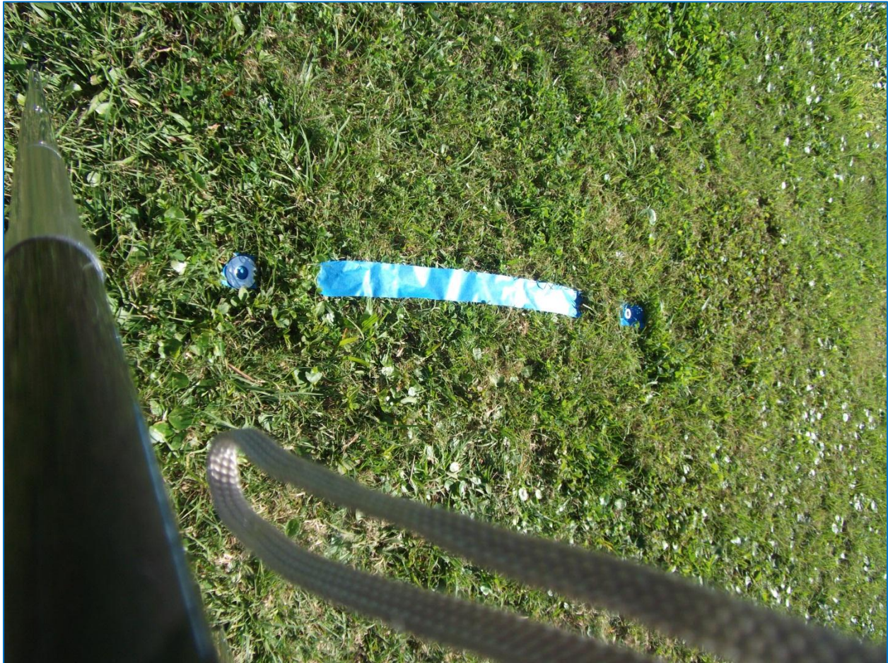
Figure 5: Two washers connected by blue tape mark true north-south line
