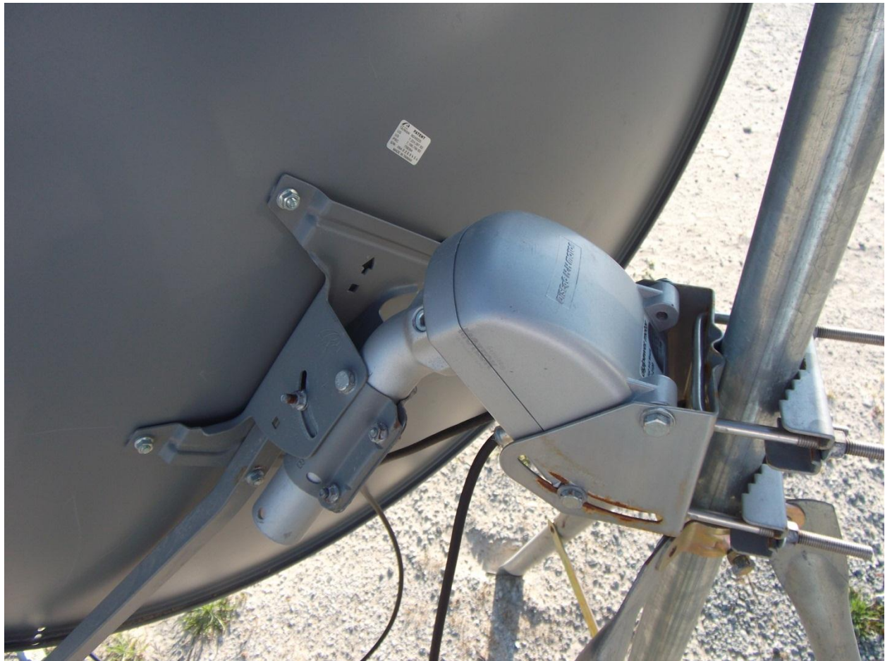
Figure 8: Install motor to mast per motor manufacturer specifications using hardware provided.
