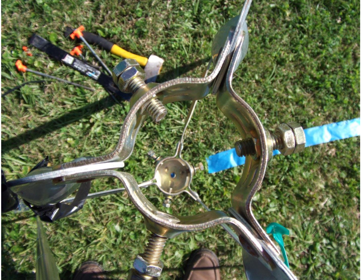
Figure 6: Mast setup exactly over mark (the washer seen in the center of mast mounting hardware).
