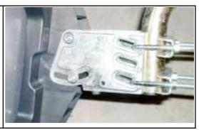
13) When adjusting these two movements, use the meter to measure the signal. Once the signal has peaked, tighten the dish elevation.
