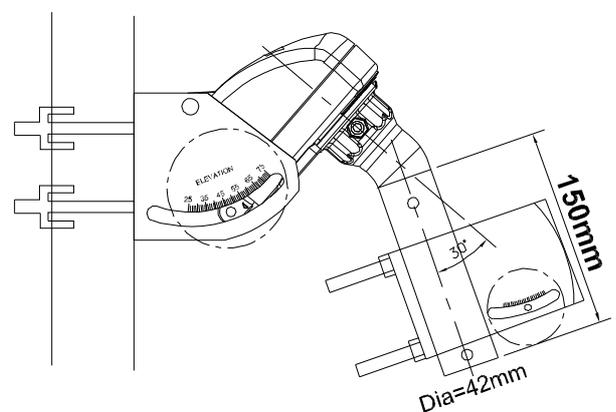
7. Move the antenna East and West using either the manual buttons on the bottom of the motor or the receiver controls verifying the reception arc is correct. If incorrect fine tune the TRUE SOUTH direction, elevation and declination angle for optimum signal strength.
