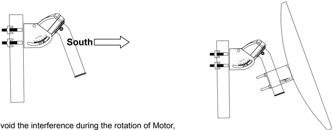
3. To avoid the interference during the rotation of Motor, please fix the coaxial cable as below.
