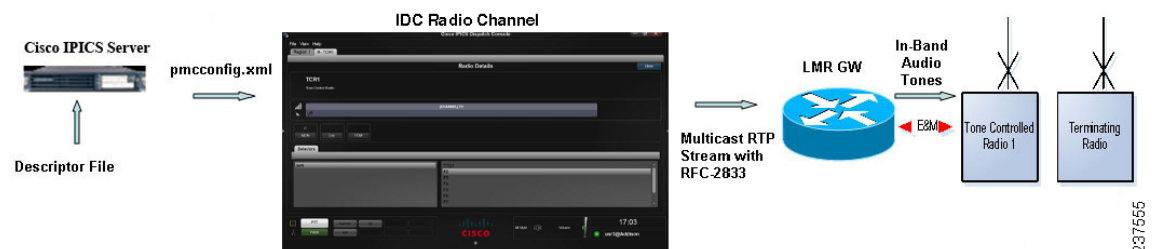
Figure 3-6 IDC Tone Remote Control Sequence
