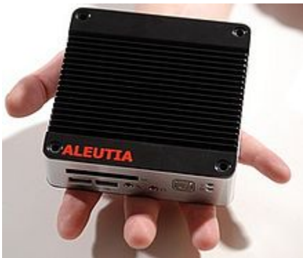
An Aleutia E3 thin client, with flash memory
