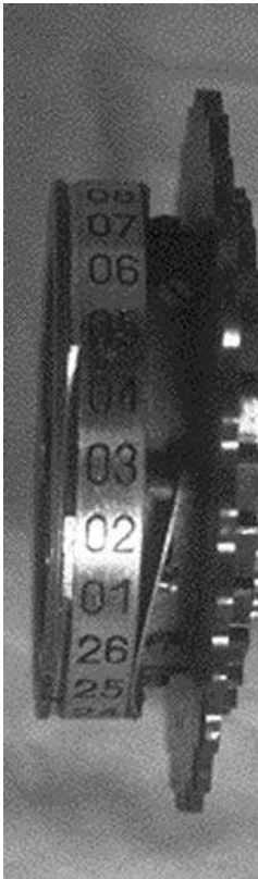
Figure 4.11 An Enigma rotor.
