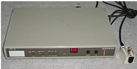
An X.25 modem once used to connect to the German Datex-P network
