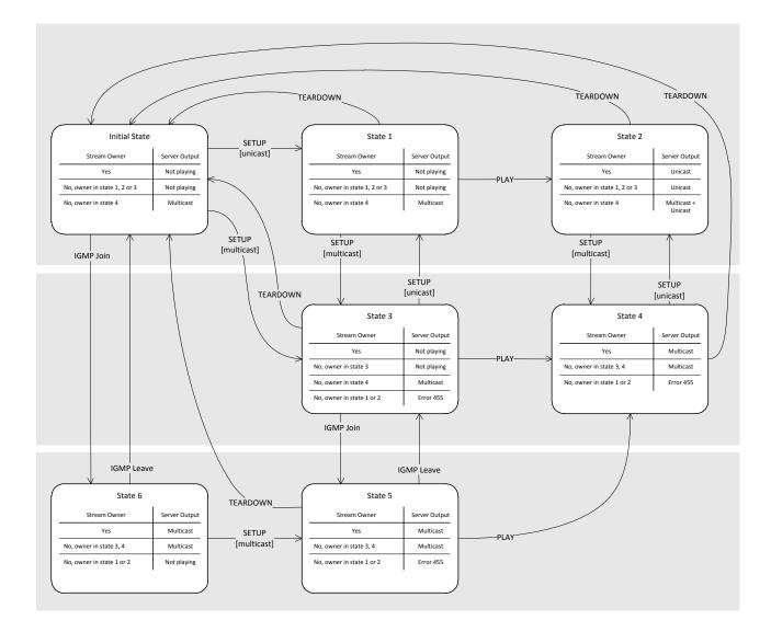
Any RTSP/IGMP method not shown in the diagram above will not modify the server output state.
