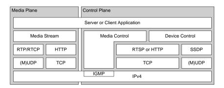
SAT>IP uses a subset of the UPnP/DLNA architecture and protocols [1] [2] and SAT>IP devices can be extended to also become DLNA devices. As an example a SAT>IP client could access live media streams through the SAT>IP protocol and access recorded media streams through DLNA.
