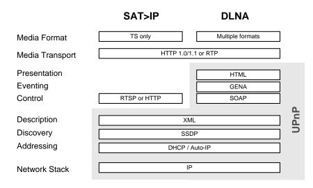
SAT>IP devices successively go through the following phases: Addressing, Discovery, Description, Control and finally Media Transport.
