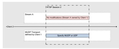
If the original transport was unicast, Client 2 may only request an additional unicast (not multicast) for itself.
